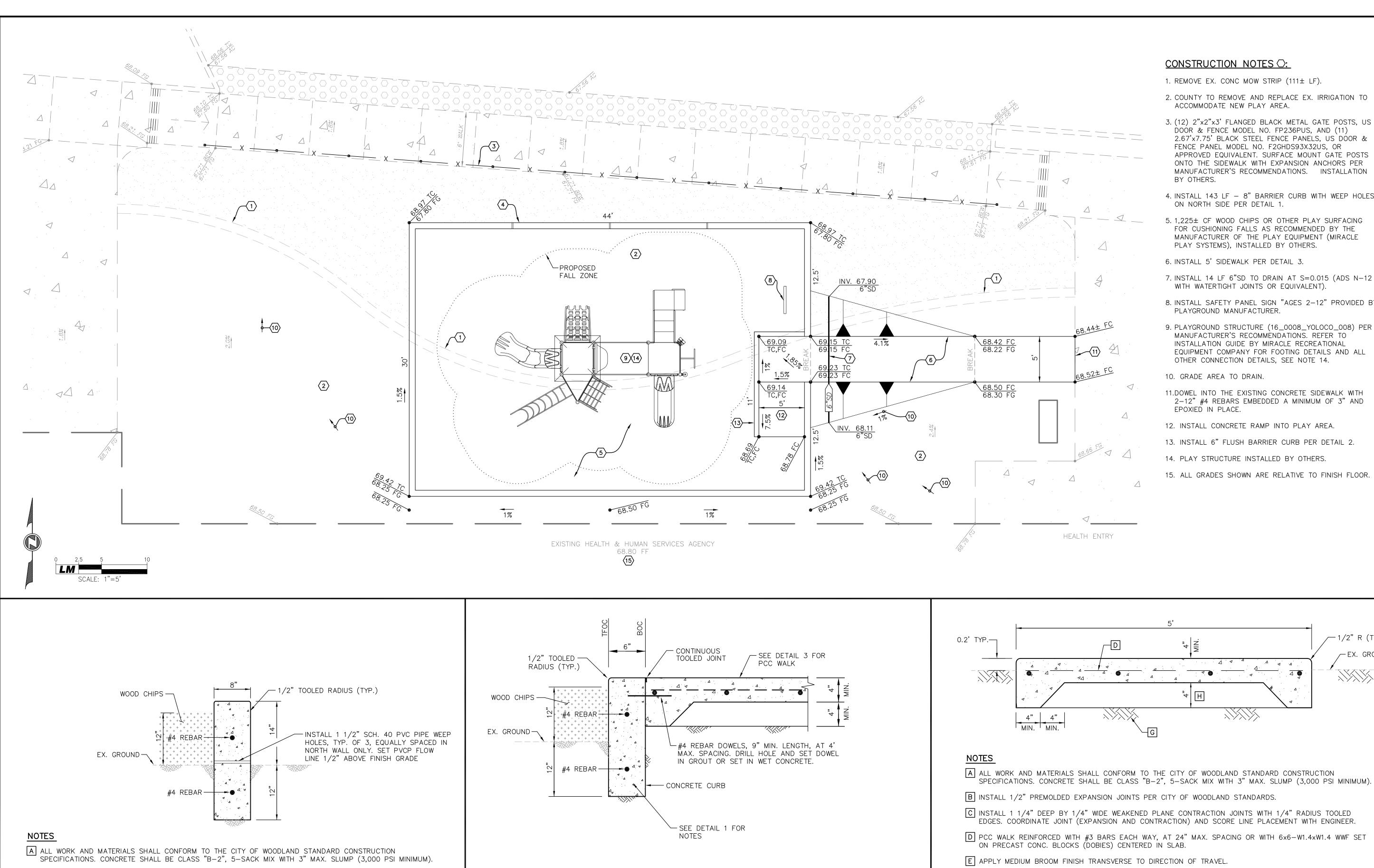
B INSTALL 1/2" PREMOLDED EXPANSION JOINTS AT 60' MAX. SPACING AND AT ALL ANGLE POINTS.
